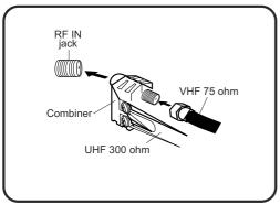
Connect the VHF 75 ohm cable and UHF 300 ohm twin-lead wire to the combiner. Attach the combiner to the RF IN jack.
